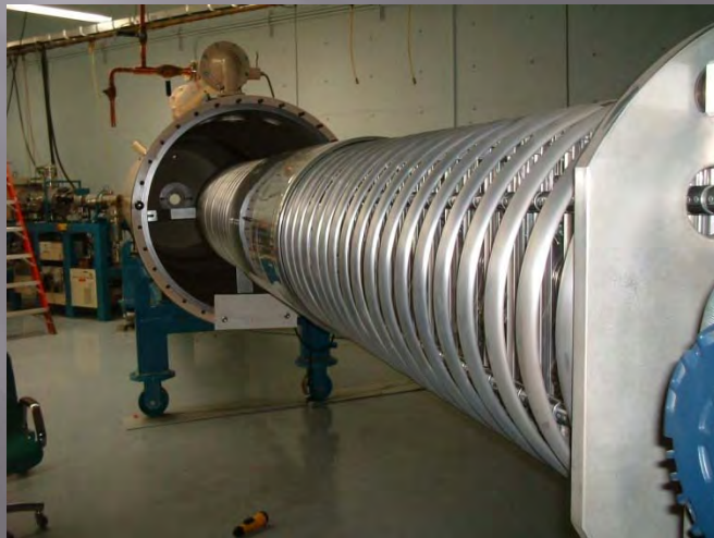
Low-energy end showing ion source and accelerator.
