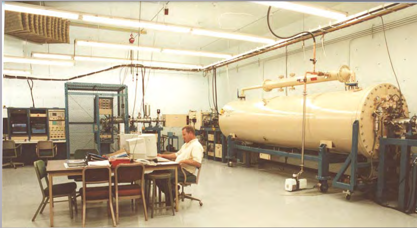
Low-energy end showing ion source and accelerator.
